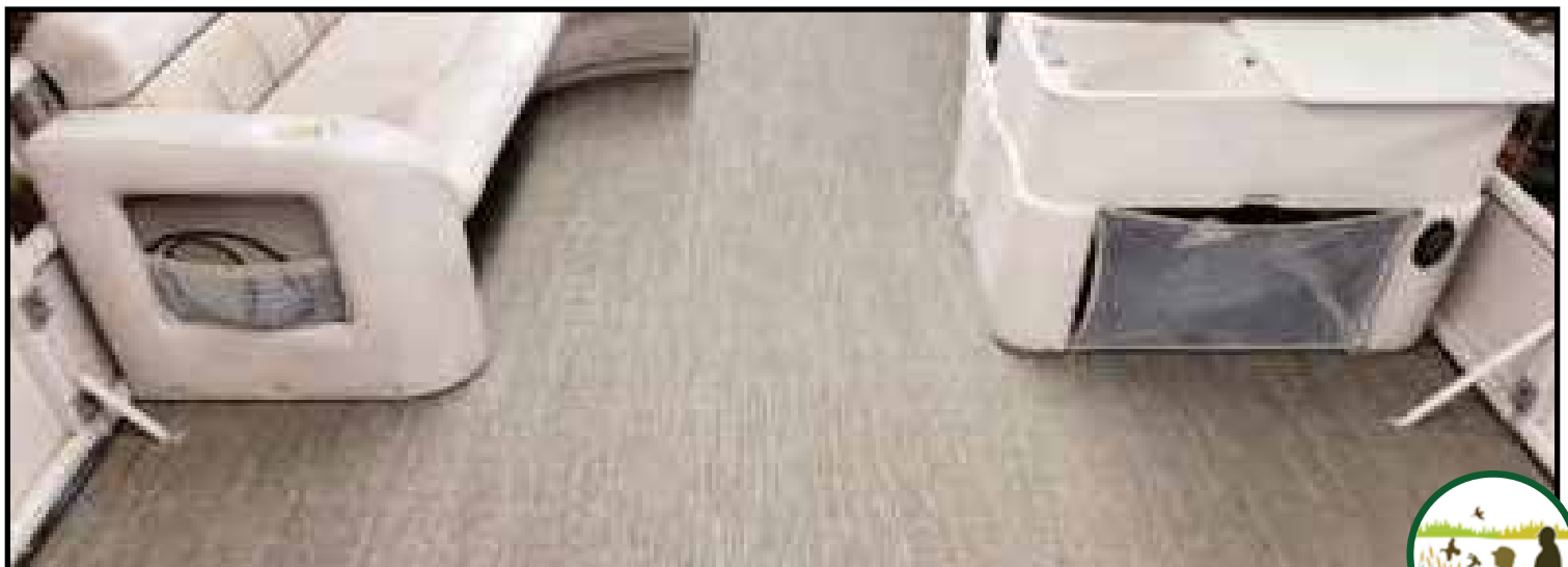
New woven flooring being applied
