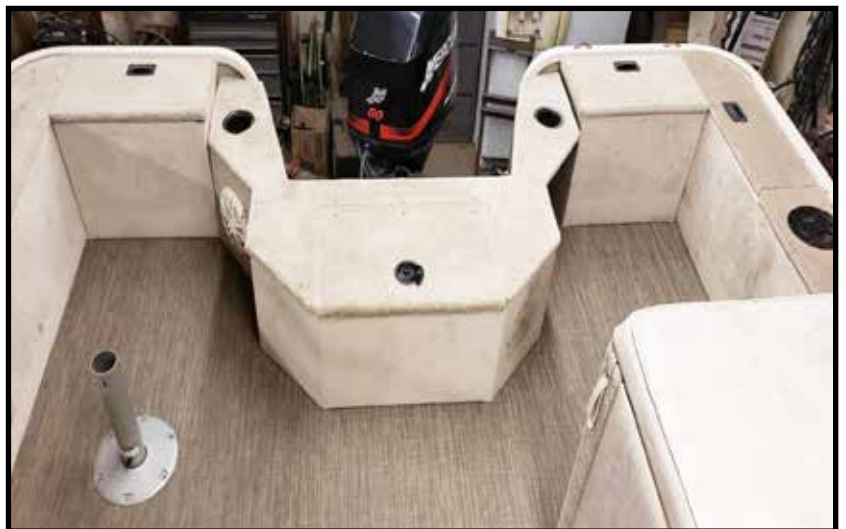
Stern of pontoon with livewell, battery and gas tank storage
